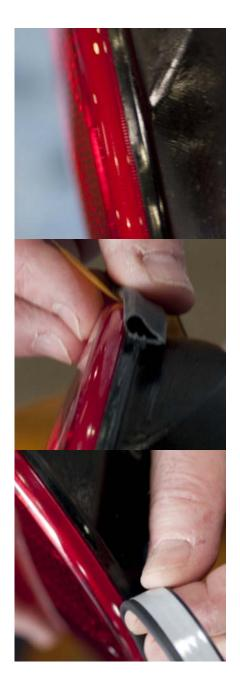
Insert Phillips head screws through tail light & place a spacer on the back. Short spacers are for the two outermost screws, long spacers are for 6 innermost screws.
